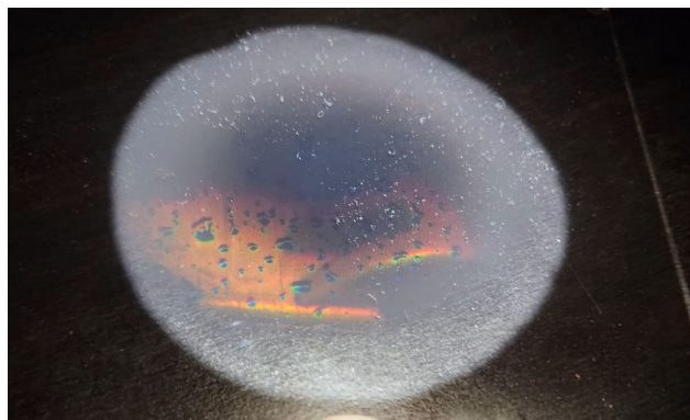
(b) Hologram observed after one week using a different laser to obtain a better viewing angle.
